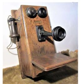
below that was the voice receptacle, which we would call the microphone today, that extended to where it could be spoken into by the user. Under that was a shelf which would be used to write notes on. The receiver or earpiece, which was used by only one ear, was hung on a cradle on the left side of the phone. This was lifted to activate the phone. The ringer was activated by a small crank on the right side of the phone.
